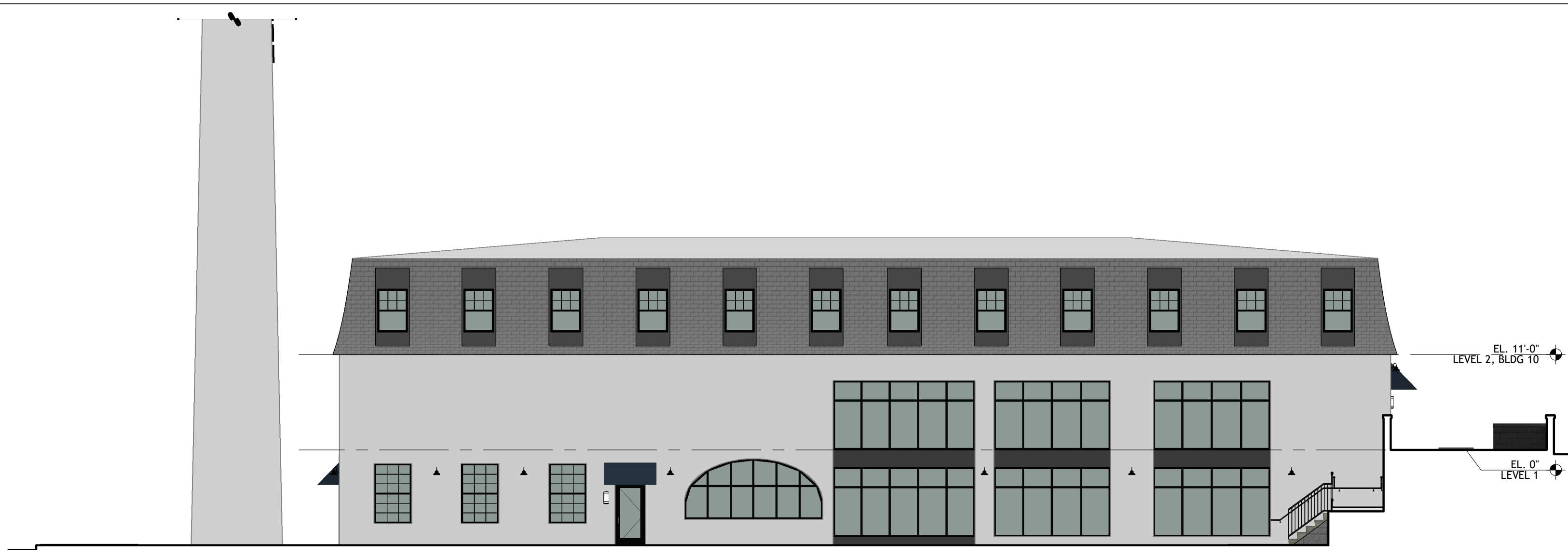
4 ELEVATION - BUILDING 10, NORTH SCALE: 3/32" = 1'-0"
